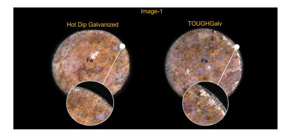
9.3 For applications that necessitate cutting the wire; the superior cathodic protection properties of TOUGHGalv provide better corrosion protection to the wire cut end.
