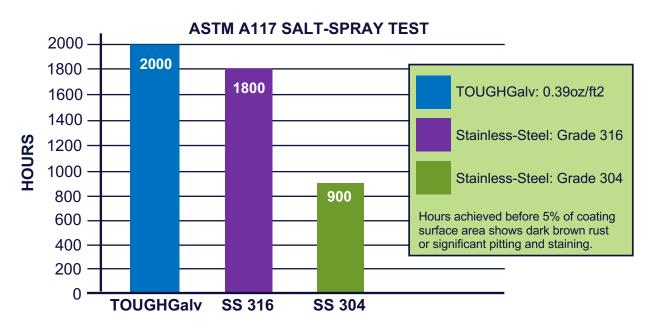
11.5 ASTM B117 testing shows both stainless-steel grades 304 and 316 exhibited pitting corrosion and significant staining. TOUGHGalv coating demonstrated superior performance than 304 and equivalent corrosion performance to 316.
